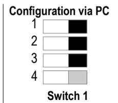
**Caution : The configuration of the parameters can be done either by DIP switch, or by software (you cannot combine both solutions).**
